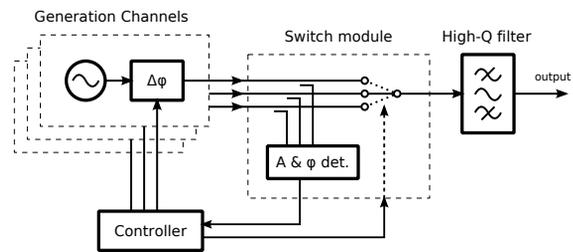
Figure 1: Simplified block diagram of the E-XFEL's MO.
