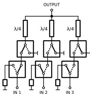
Figure 4: Used topology of microwave SP3T absorptive switch constructed from six DPDT switches.
