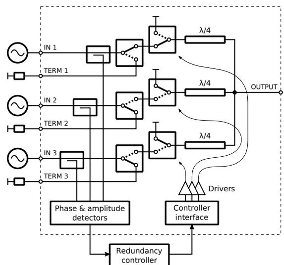
Figure 2: Simplified block diagram of the switch module.
