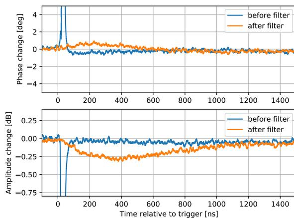
Figure 6: Phase and amplitude variations during switching in near-ideal conditions.
