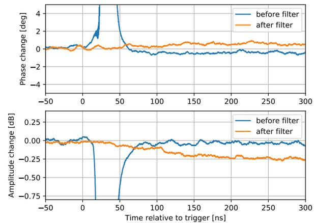
Figure 7: Phase and amplitude variations during switching in near-ideal conditions (cropped to the first 300 ns).
