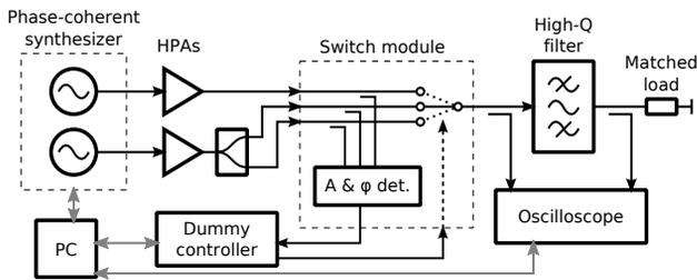
Figure 5: Block diagram of the test setup.
