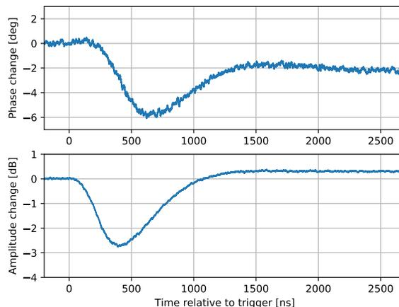
Figure 10: Phase and amplitude variations during switching in simulated failure response.
