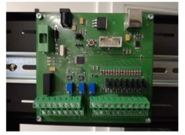
Figure 1: General purpose measuring board Board51.
