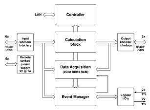
Figure 1: PEPU functional block diagram.
