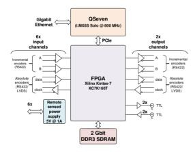
Figure 2: PEPU implementation block diagram.
