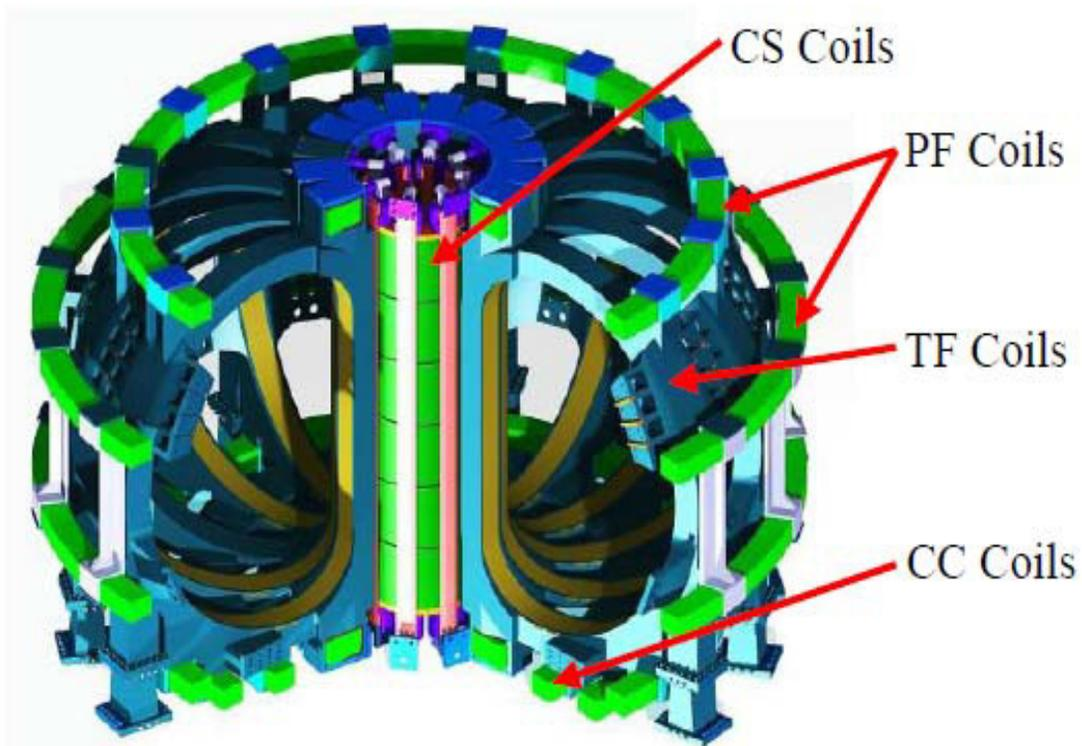
Figure 1: Magnets system of CFETR.
