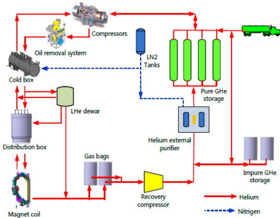
Figure 2: Cryogenic system of CFETR TF coil test facility.
