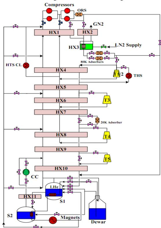
Figure 3: PFD of helium refrigerator.
