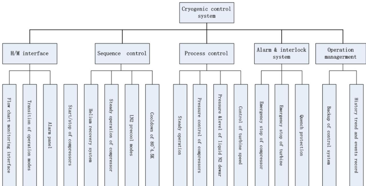
Figure 5: Software structure of cryogenic control system.
