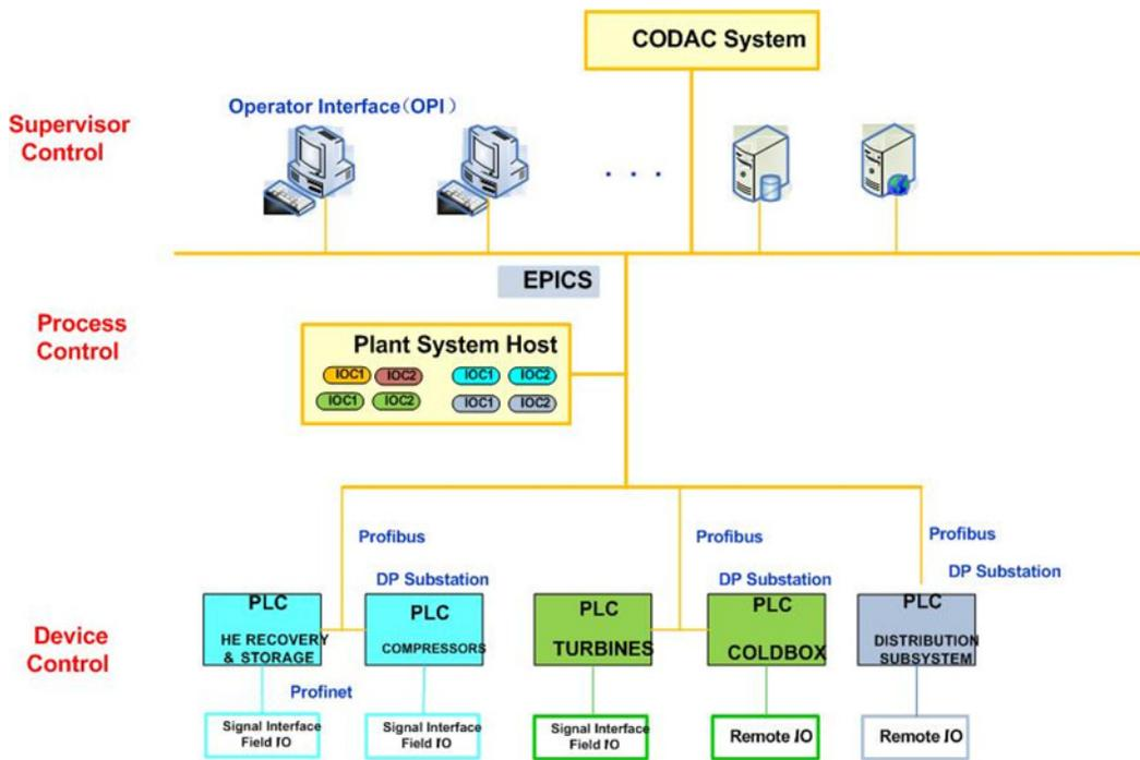
Figure 4: Structure of cryogenic control system.
