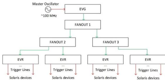
Figure 4: Basic structure of SOLARIS timing system.
