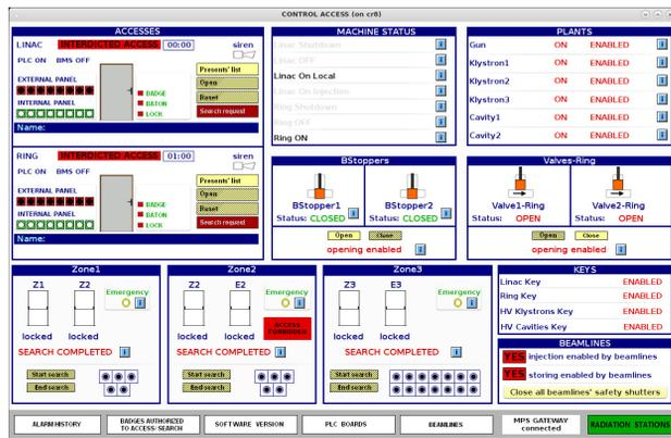
Figure 3: Personal Safety System GUI.
