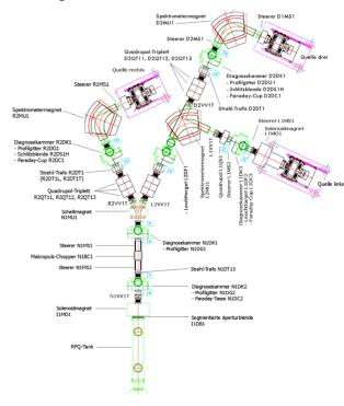
Figure 2: New LEBT with three ion sources.
