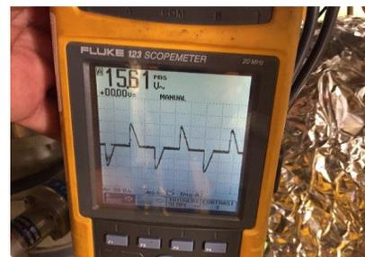
Figure 9: Filament Voltage Oscillogram.
