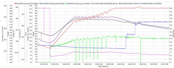
Figure 11: Archived data from successful klystron bakeout.
