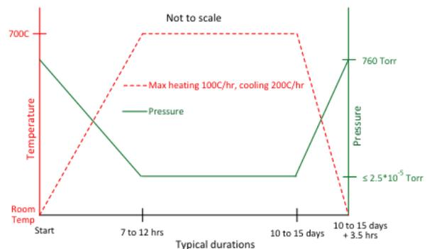
Figure 2: Example vessel temperature and pressure vs. time profile (not measured data).
