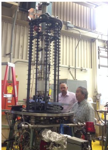
Figure 1: Bake station 5 with oven shell removed (device in center is klystron tube awaiting bake-out).
