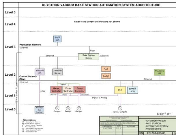
Figure 6: Bake station network architecture.
