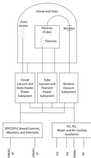
Figure 4: Generalized hardware architecture.
