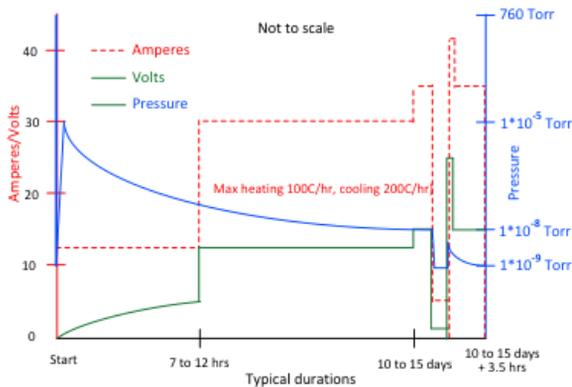
Figure 3: Example klystron filament voltage and current profile (not measured data).
