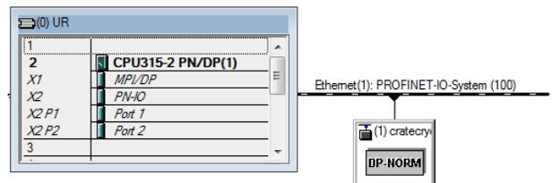
Figure 10: Siemens© Step 7 programming environment and CRATE configuration.
