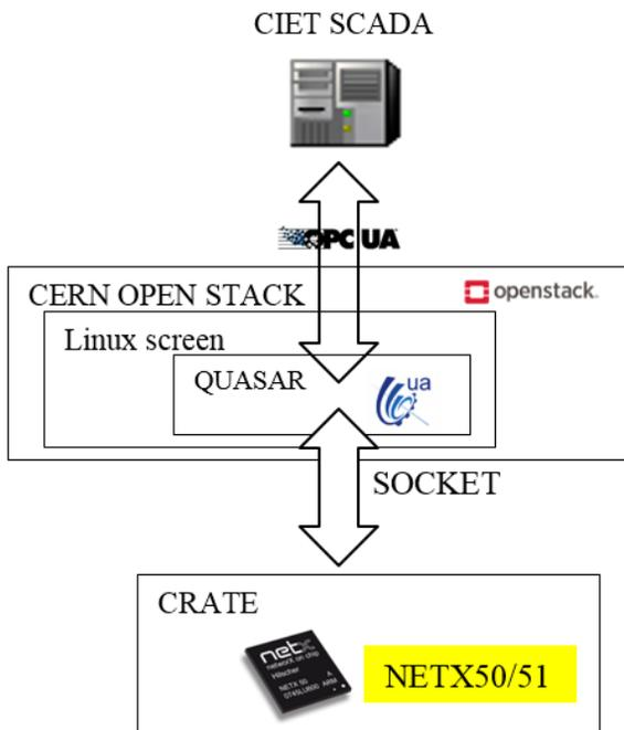
Figure 14: OPC UA™ communication using the socket.
