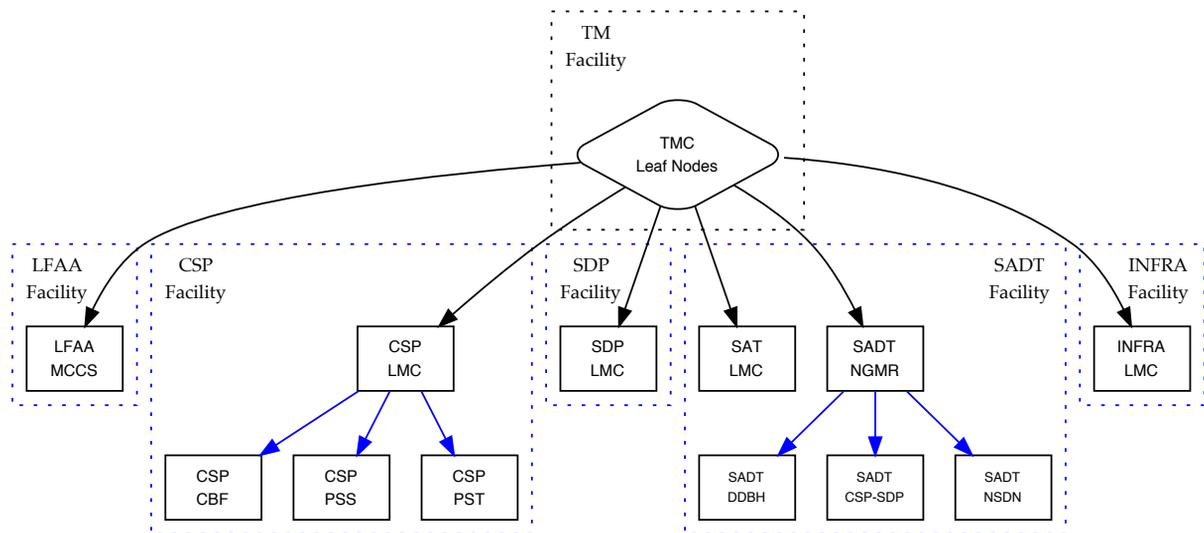
Figure 9: High-level overview of the SKA1-Low Facilities. The LFAA MCCS exposes control to a very large hierarchy of devices, not shown here. Compare with Fig. 8.
