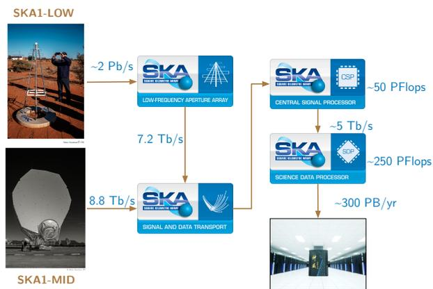
Figure 6: Notional data flows and computational intensity required by the SKA1 telescopes, with shared Central Signal Processor (CSP) and Science Data Processor (SDP) for convenience.
