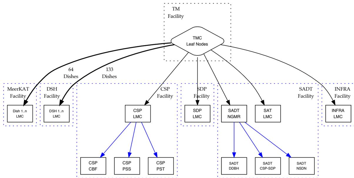
Figure 8: High-level overview of the SKA1-Mid Facilities. There are 133 Facilities for each of the SKA1-Mid dishes, while there is only one facility for the 64 MeerKAT dishes. Compare with Fig. 9.
