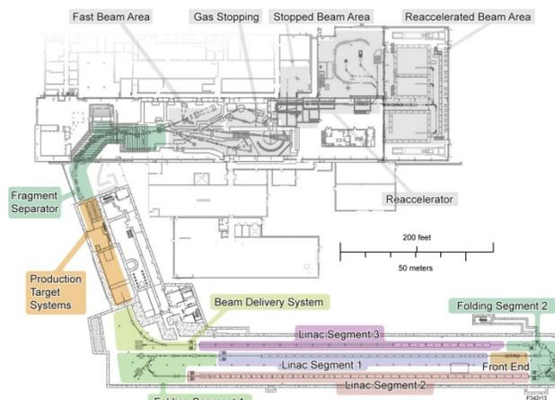
Figure 1: Schematic layout of the FRIB (colored areas) and existing infrastructure (gray).
