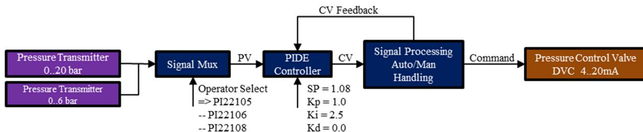
Figure 2: Example PIDE implementation for FRIB cryoplant.
