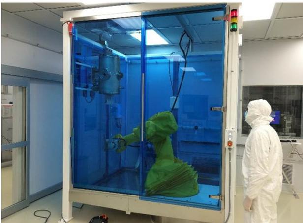
Figure 4: Robotic HPR system installed at FRIB.
