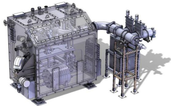
Figure 6: Lithium charge stripper test stand.
