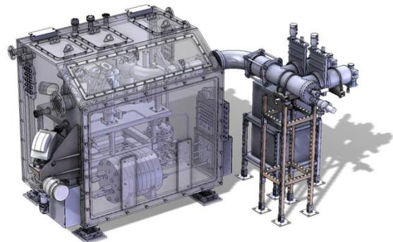
Figure 6: Lithium charge stripper test stand.
