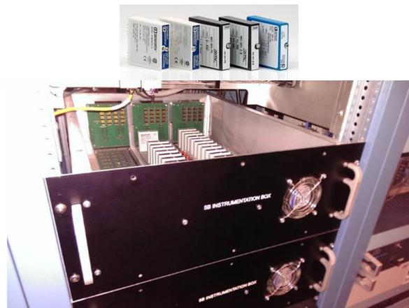
Figure 5: Instrumentation box utilizing 5B modules.
