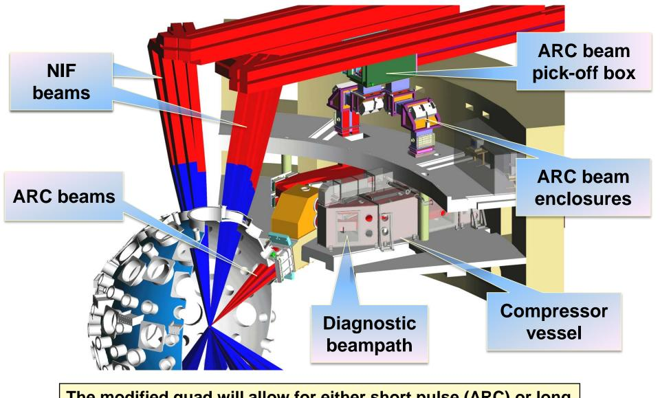
The modified quad will allow for either short pulse (ARC) or long pulse (NIF) operations
