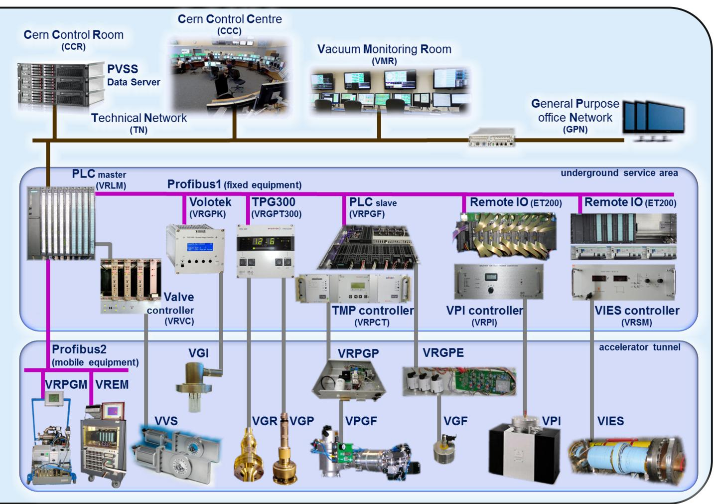
Hardware: upgraded to a PLC-based architecture with Siemens<sup>™</sup> S7 and PVSS<sup>®</sup> (now called WinCC<sup>®</sup>-OA).
