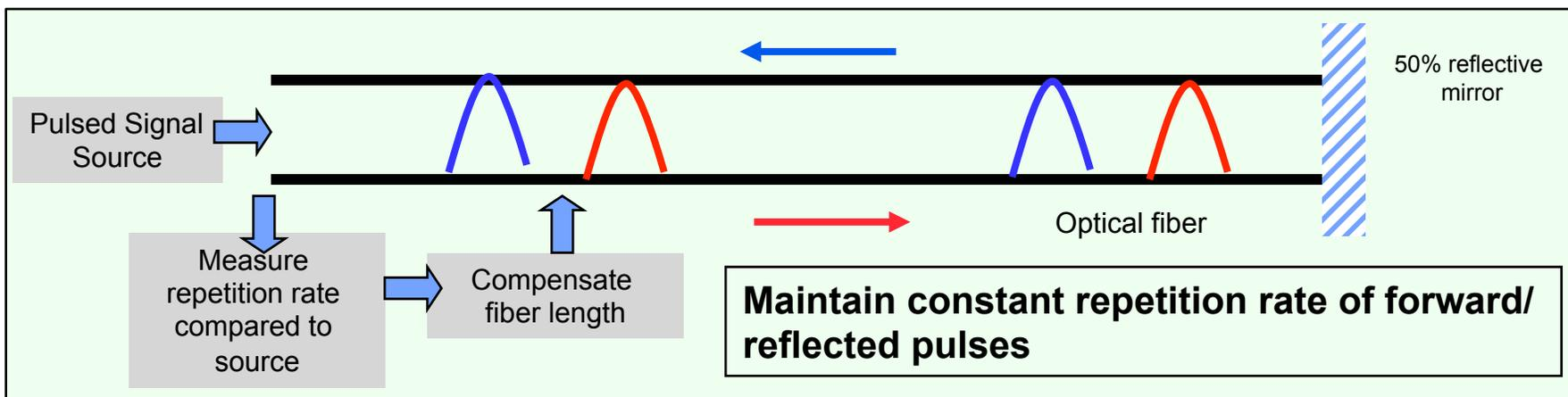
Correction BW limited to R/T travel time on fiber (e.g. 1 km fiber gives 100 kHz)
