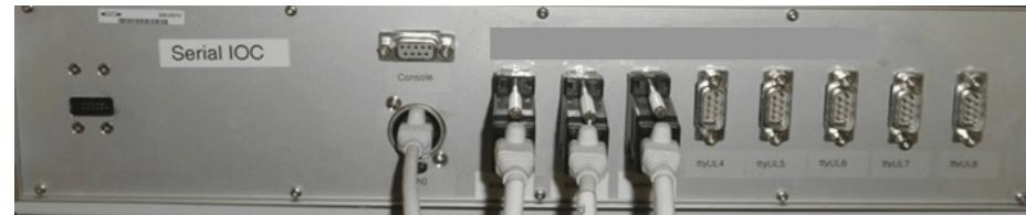
**Serial (RS232) devices are mostly handled by custom made embedded controllers based on Virtex-4 FPGA**
