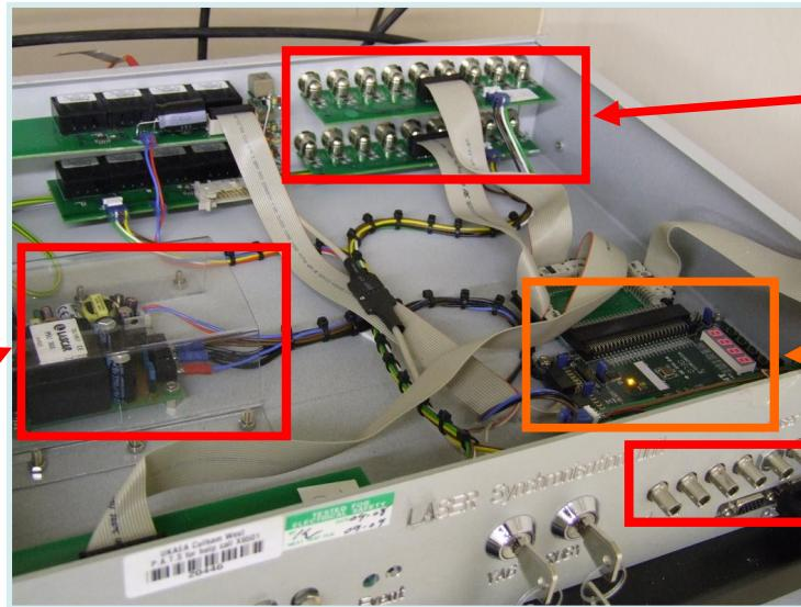
BNC 50 Ohm driving signals to each of the 8 lasers
