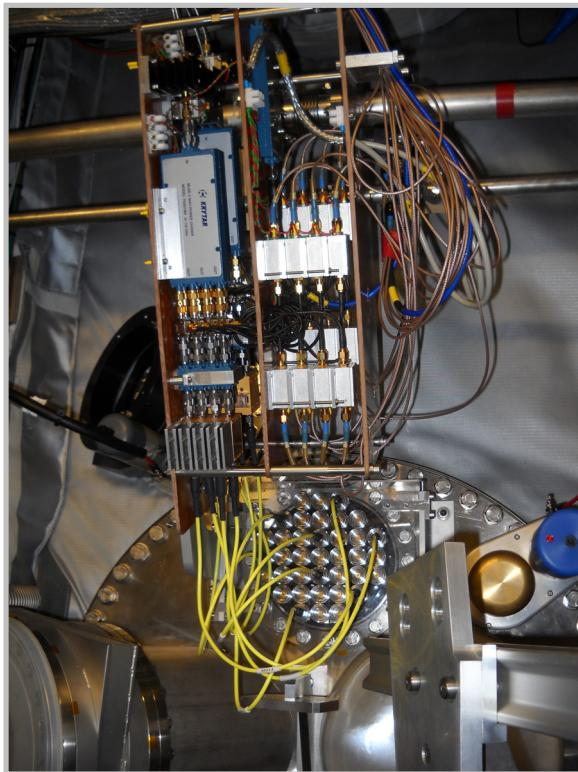
**Ultra high performance FPGA system for acquiring and analysing 6-40 GHz microwave radiation emitted by the plasma.**
