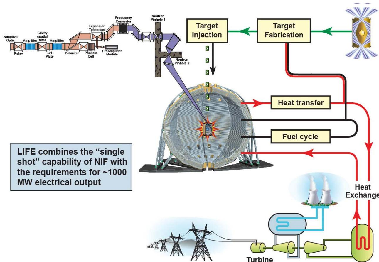
LIFE combines the “single shot” capability of NIF with the requirements for ~1000 MW electrical output
