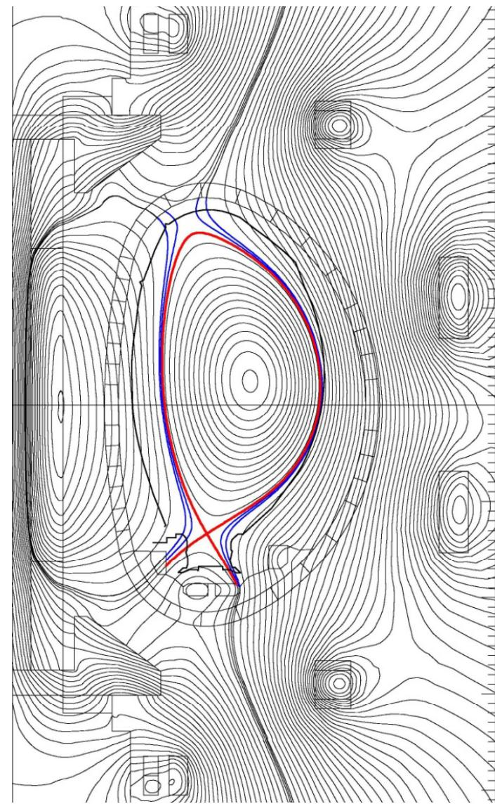
Tokamak → Plasma within a **torus** shaped vacuum vessel → **doughnut**.
