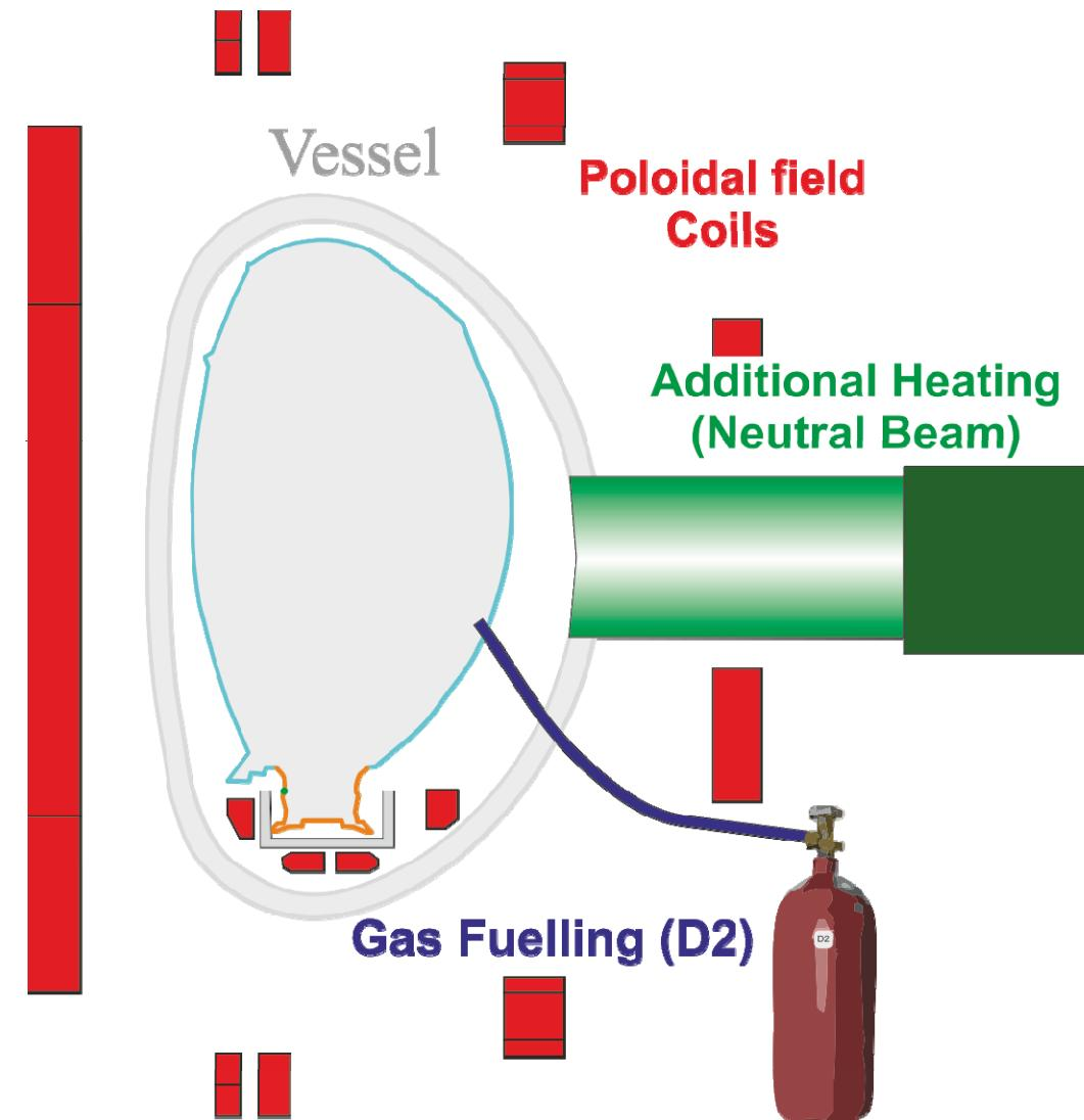
*The Central solenoid creates an electric field. GAS is added and ionised → plasma.*
