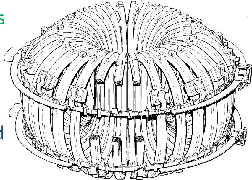
The TF coils create a *toroidal* field which helps avoiding instabilities.
