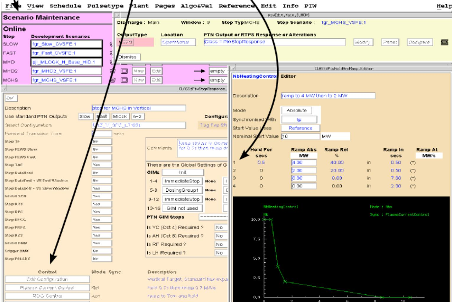
The screenshot displays the 'Scenario Maintenance' window with a list of development scenarios for different stop types (SLOW, FAST, MHD, MHD2, MCHS). The 'NbHeatingControl' editor is open, showing a description 'ramp to 4 MW then to 2 MW' and a table of control parameters.
