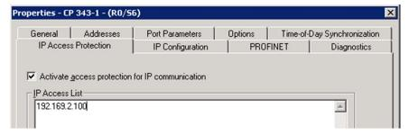
► Enable PLC intrusion detection
