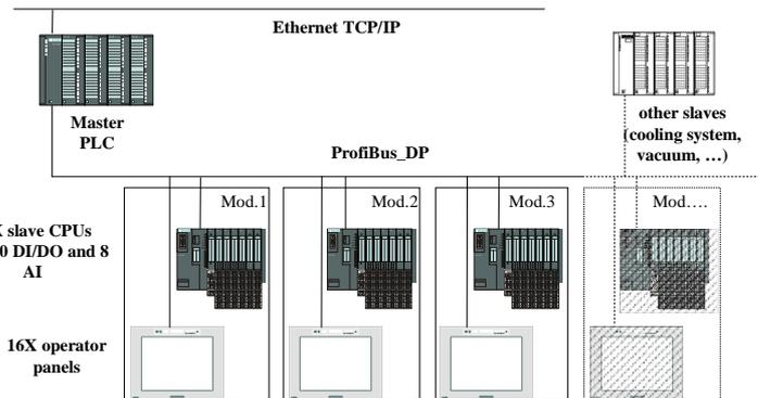
The block diagram of the linac RF plants interlock system.
