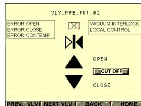
Fig.2: The vacuum valve control page
