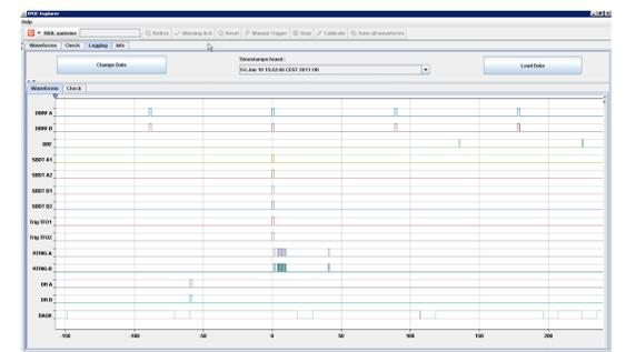
**Logic analyser function** to perform after each dump a check of the correct sequence of triggering and re-triggering pulses, the correct delays between the different signals, the sanity of the signals, the correct frequency and phase offset between distributed and internally generated re-phased beam revolution frequency
