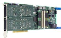
Based on a PCI 32 bit 125 MS/s digital I/O module from SPECTRUM with acquisition software running on a LINUX front-end
