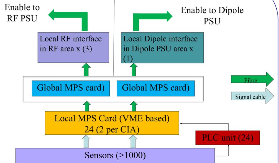
Plant sensors include:- Thermostats, PT100's, Flow meters, Valve position limit switches, Vacuum Gauge level set-points, Beam position Sensors, Beam Stability Sensors and Front End & Beamline Healthy (Beamline masked by Front End).
