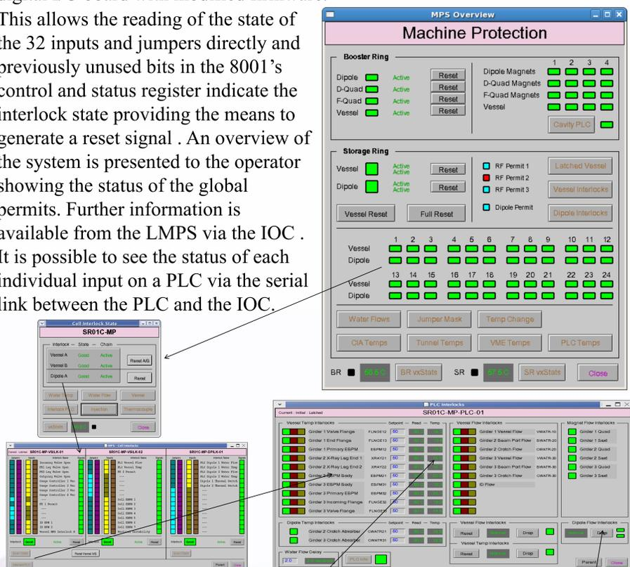
The PLC screen allows the operator to change the thermal trip points and add filtering to water interlock inputs to allow dips in water flow to be ignored. It also features a Beam trip test button which allows for automated testing of each sector of the MPS after a shutdown.
