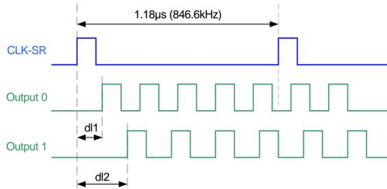
The two clocks high and low levels ratio can be adjusted by the user. This allows odd frequency division. For example for a RF / 17 division, the user can configure the output for 8 high levels and 9 low levels (8 + 9 = 17). Of course, he can also configure 1 high level and 16 low levels, or 16 high levels and 1 low level.
