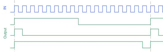
Clock outputs are automatically synchronized to the storage ring clock. Thus the offsets from the electron bunches are always the same.
