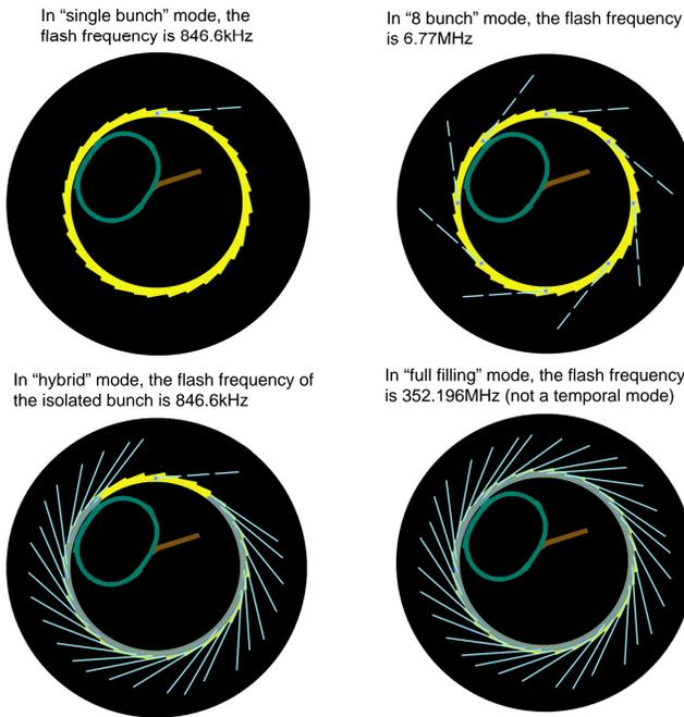
Figure 3 : Synchrotron SOLEIL filling modes
