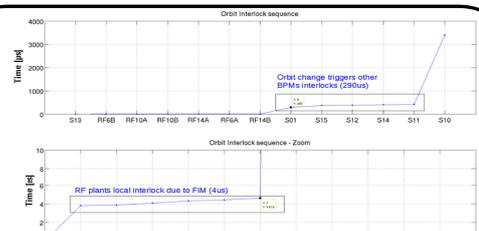
Complete sequence of one BPM interlock timestamped with the Fast Interlock System: a orbit interlock is detected in one BPM in SR in sector 13 and timestamped. The Fast Interlock system induces a shutdown of the six RF Plants 4µs later and that leads to a loss of the orbit in the rest of BPM sectors after 290µs.
