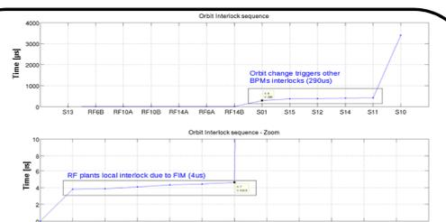
Complete sequence of one BPM interlock timestamped with the Fast Interlock System: a orbit interlock is detected in one BPM in SR in sector 13 and timestamped. The Fast Interlock system induces a shutdown of the six RF Plants 4µs later and that leads to a loss of the orbit in the rest of BPM sectors after 290µs.
