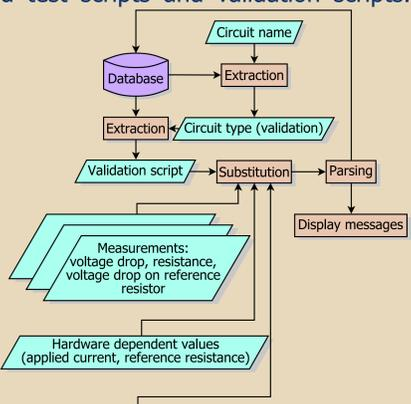
Figure 5. Measurement results validation process.
