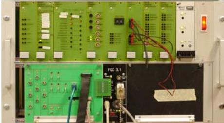
This chassis allows the simulation of the power converter signals, the connection of debugger interfaces for the 3 processors, the use of test points and measurement of analog signals.
