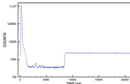
Time between BGO (start) and Ge (stop), measured for  $^{22}\text{Na}$  source in pair spectrometer mode
