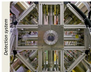
**Scientific goal:** to measure the  $e^+e^-$  pair-production cross-section close to the 1022 keV threshold.
