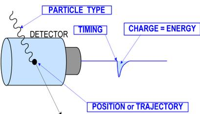
The front-end electronics must provide precise information about amplitude, time, detection position and possibly pulse shape.
