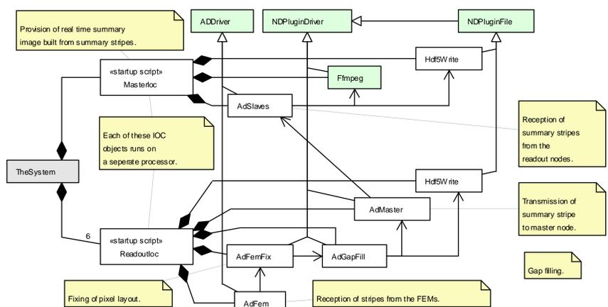
The embedded software is based on EPICS using the area detector module. Above is a UML diagram showing an overview of the data path software; the classes ADDriver, NDPluginDriver and NDPluginFile are area detector base classes supplied by the module library.
