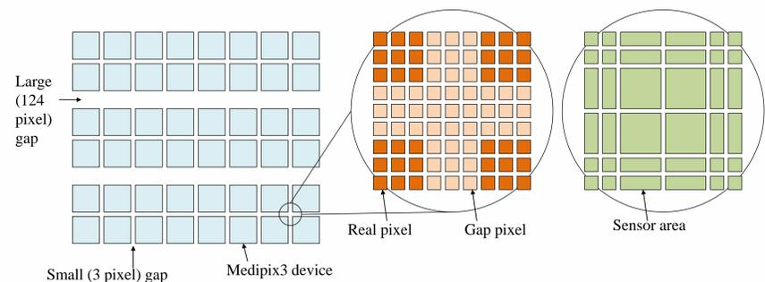
The gaps between the adjacent Medipix3 chips are required to be filled, either by a constant value or by interpolation between the pixels surrounding the gap. The chip layout and gap details are shown above. The class responsible for the work is AdGapFill (see Software Architecture).
