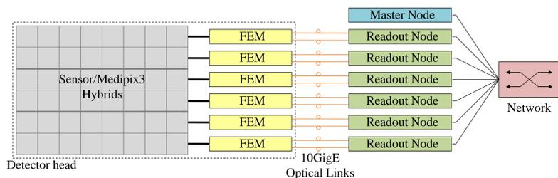
The hardware architecture consists of a sensor assembly, a number of front-end modules (FEMs) and a cluster of read-out node PCs.
