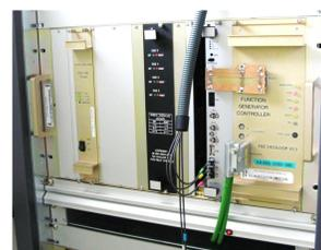
Function Generator/Controller regulating magnetic field with the POPS converter
