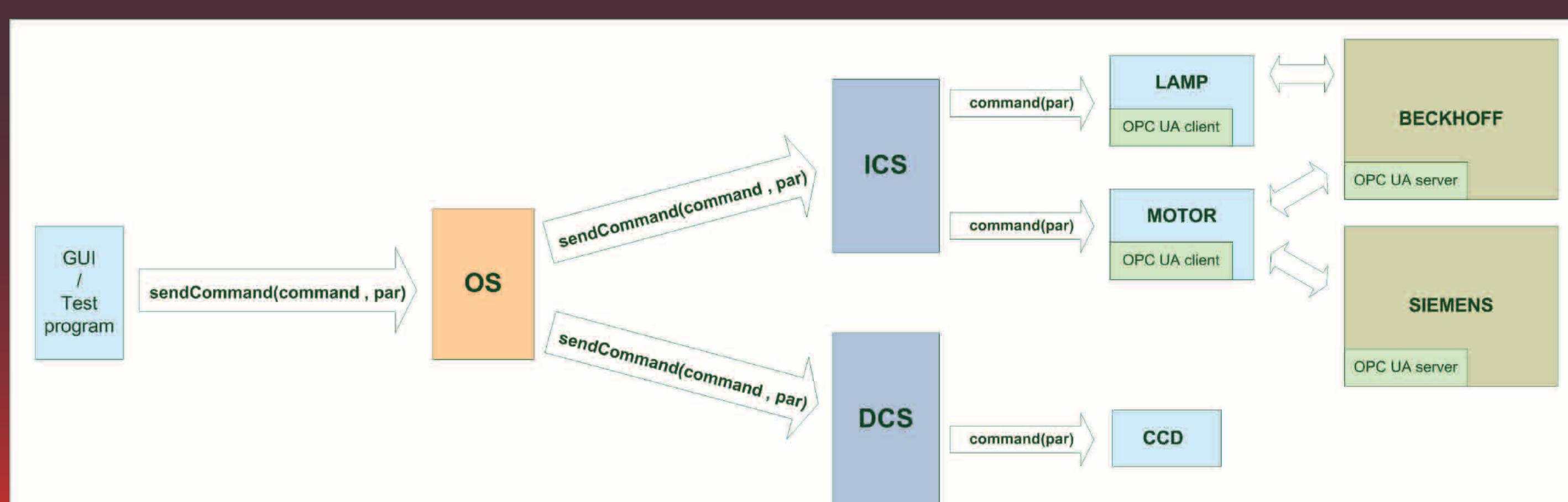
The prototype software infrastructure is based on the ACS (ALMA Common Software) framework. The ACS philosophy is to model the system as a set of collaborating components located inside one or more containers (Component/Container paradigm).
