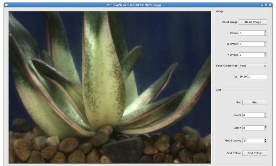
The areaDetector module provides a common interface for all supported 2d detectors. Integrating the camera into areaDetector allows image processing and analysis plug-ins to be chained together at runtime, such as the NDStats plug-in for statistics, or the ffmpegServer plug-in to provide a compressed mjpg stream for visualisation
