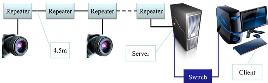
Gigabit Ethernet cameras allow up to 100m data transfer lengths, with greatly simplified cabling. Connecting additional cameras at a later date is also simpler
