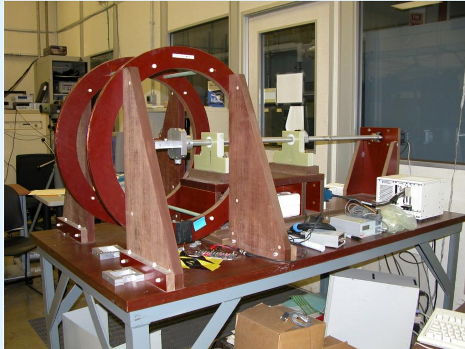
Figure 1. Helmholtz coil magnet measurement system.
