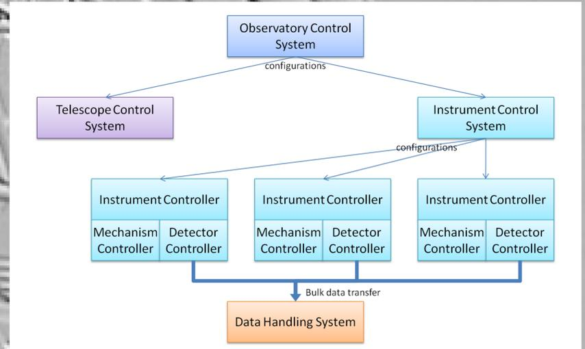
Configurations are sent from the OCS to the TCS and ICS. The ICS coordinates the start and stop of data collection in the active instruments.
