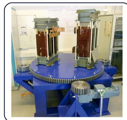
Fig. 3: MST prototype drive test stand
