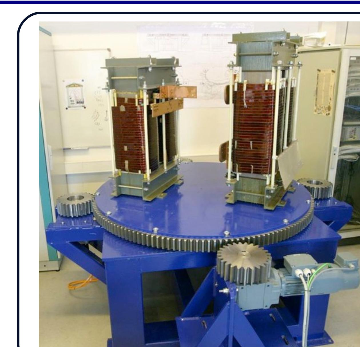
Fig. 3: MST prototype drive test stand
