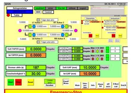
The graphical user interface consists of main control window, intersection control, alarm display, axes status and system information.
