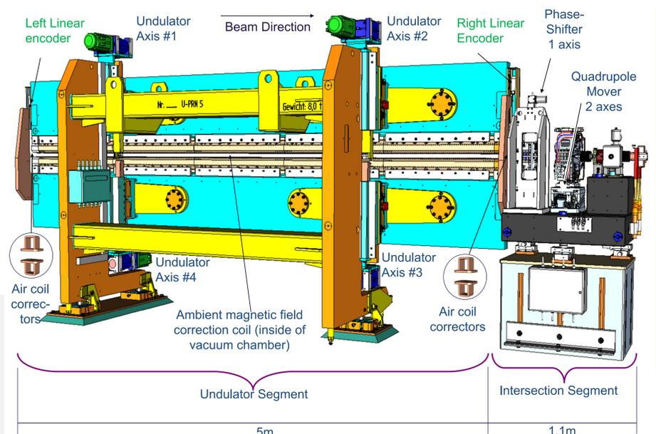
Control components of an undulator cell
