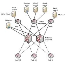
Figure 5: Global control net. The core switch is redundant to avoid shutdown of whole system. And links to core switch is also redundant. The failure of other switch only impact local sub-system.
