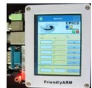
Figure 7: IOC based on ARM.
