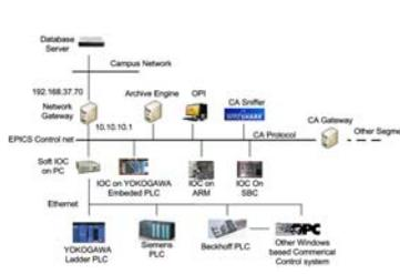
Figure 3: EPICS system architecture. In this figure, all components have been integrated into EPICS are shown.
