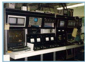
Control Room circa 1985. The right (grey counter) is the accelerator control system including the original Booster and added ATLAS sections. The left (white counter) is the added beamline control system.
