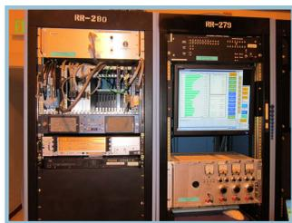
The distributed Cryogenic Monitoring system has been updated from a distributed CAMAC system to a VME system.
