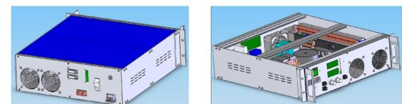
The main part of the control subsystem is a rack-mounted industrial PC. It performs all interactions with power supplies such as generation of reference signals, monitoring of the power supply output current and status controlling.
