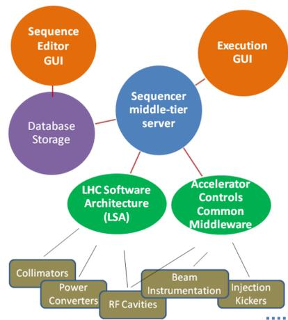
Figure 1: LHC Sequencer Architecture.
