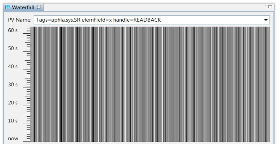
Figure 5: WaterFall plot for all x field readback channels in storage ring.
