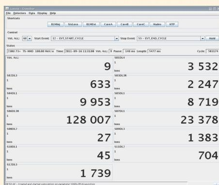
Most of the experiments and users of beams need to know the amount of particles on their target. This information is provided by the counter tool. It shows the integral sum-up of all particles per cycle.
