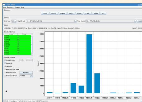
The spill structure tool (picture below) provides a setting for beam loss monitors of all 12 synchrotron sections at the SIS18 at GSI to observe all potential beam loss locations simultaneously. Here the count rate as a function of time gives further information of the type and moment of beam loss.
