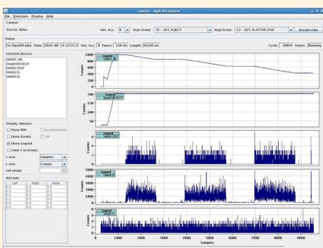
Another example of the spill structure analysis is given below. With end of the acceleration flattop (1st graph, transformer) the losses at the extraction section rise significantly (2nd graph, BLM). The losses at the electrostatic septum are low (3rd graph, BLM)
