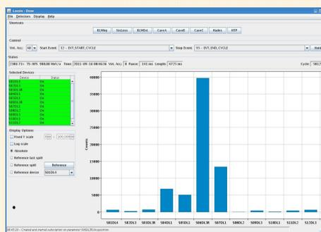
The spill structure tool (picture below) provides a setting for beam loss monitors of all 12 synchrotron sections at the SIS18 at GSI to observe all potential beam loss locations simultaneously. Here the count rate as a function of time gives further information of the type and moment of beam loss.
