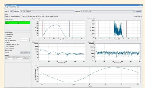
To optimize the beam e.g. the particle distribution within a spill some expert tools were developed. First, the cross analysis tool (picture above) provides on the one hand FFT analysis for deeper understanding of selected signals and on the other hand a way to cross correlate two signals on a time base. Here a synchrotron transformer is correlated with a BLM at the extraction line. Good correlation can be seen for the time of the extraction approx. 0.7s shifted to the right.
