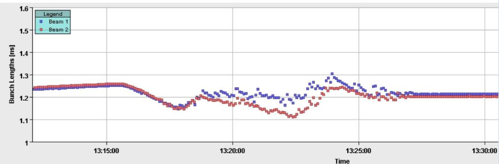
Fig. 5. Four-sigma bunch length evolution during a ramp with the blow-up system set for a 1.2 ns target. Start of ramp at  $\sim 13:16$ , end at  $\sim 13:27$ .
