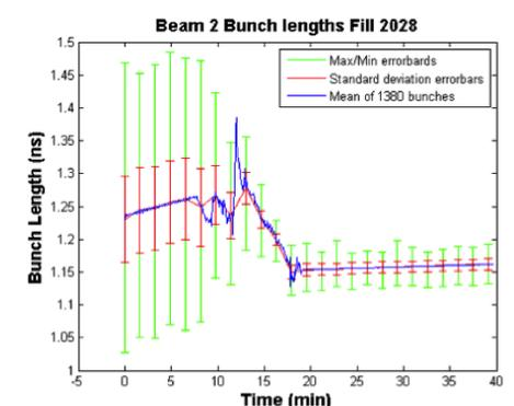
Fig. 7. Statistics on bunch length (mean, min, max and standard deviation error bars) measured by the BQM during the ramp.
