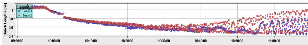
Fig. 1. Bunch length during ramp. The longitudinal emittance is too low ( $\approx 0.4$  eVs). The bunch becomes unstable (quadrupole oscillations).
