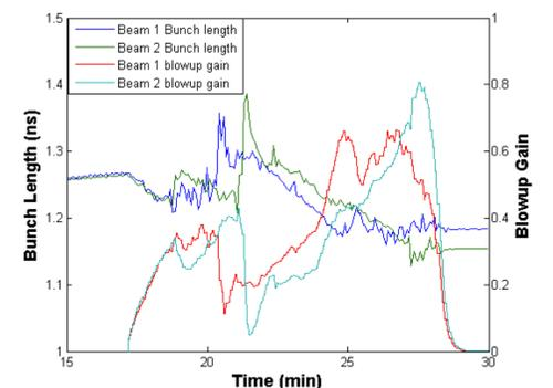
Fig. 6. Bunch length (mean over 1380 bunches/beam) and excitation (blowup gain) during the ramp.
