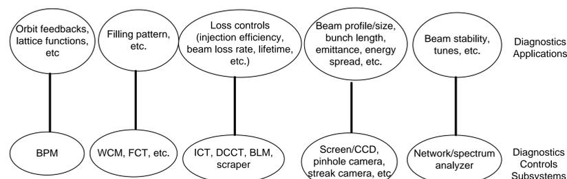
Figure 2: Diagnostics Control Subsystems and Applications
