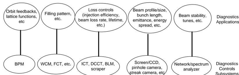
Figure 2: Diagnostics Control Subsystems and Applications
