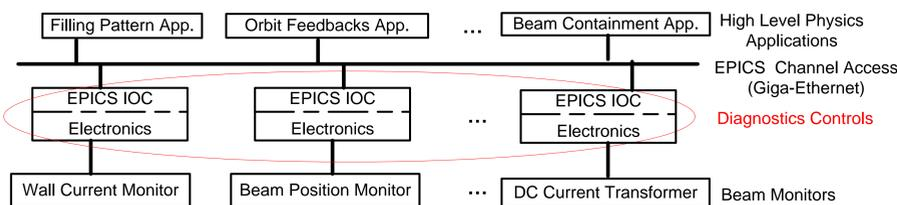
Figure 1: NSLS-II Beam Diagnostics & Control Systems
