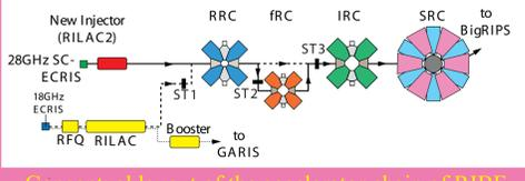
Conceptual layout of the accelerator chain of RIBF
