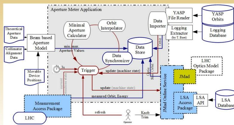
Figure 2: Aperture Meter components and their interaction for  $a_z(s)$  calculation.
