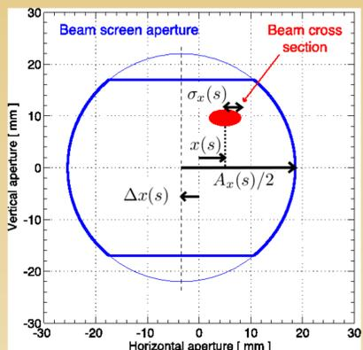
Figure 1: Beam screen aperture with relevant aperture definitions (horizontal plane)
