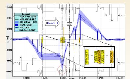
Figure 5: Beam 1 Horizontal, beam trajectory in mechanical aperture at max. bump excursion during triplet scan in IP5 (CMS)
