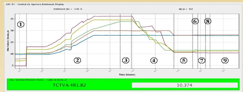
Figure 3: Minimal aperture evolution for beam 2 vertical plane over the operational cycle. The primary and secondary collimator positions are not taken into account.
