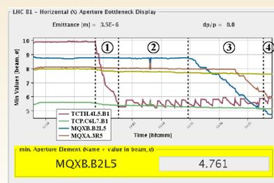
Figure 4: Beam 1 Horizontal, minimal aperture evolution during triplet scan in IP5 (CMS)
