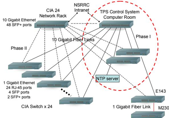
Figure 2: TPS control network – baseline plan.
