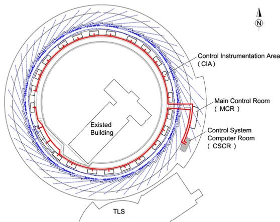
Figure 3: Fiber distribution for control computer network.
