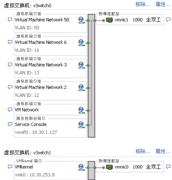
Figure 2: VLAN configure in virtual switch.
