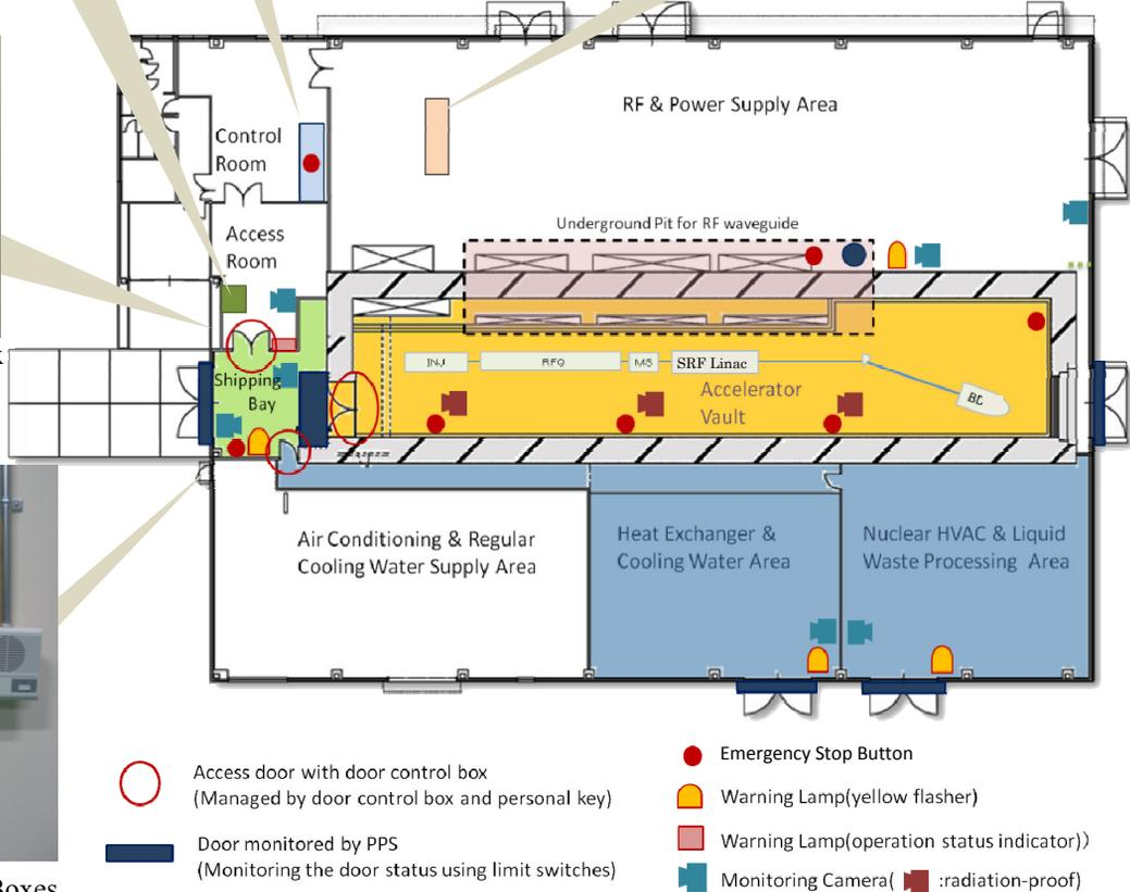
Figure 2: Radiation controlled area and Layout of main equipment for the PPS.
