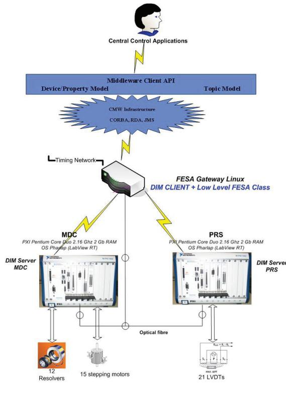
Figure 1: Architecture of the LHC collimator control system.
