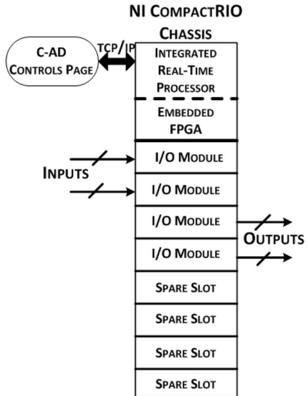
Figure 3: Block diagram for the current layout.
