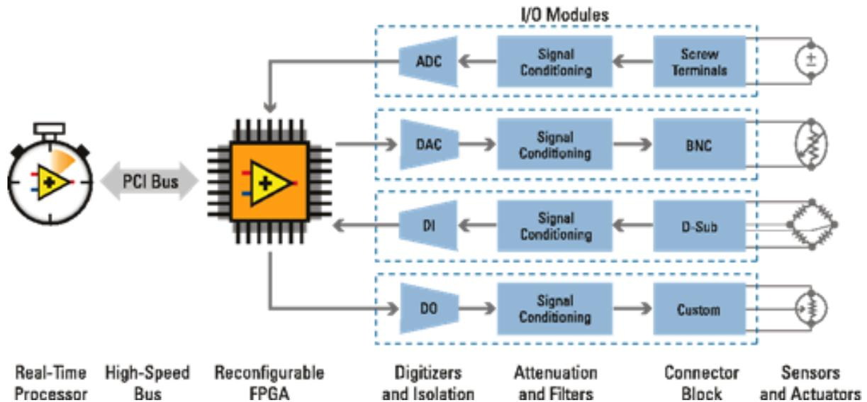
Figure 2: Block diagram showing a generic CompactRIO architecture [2].
